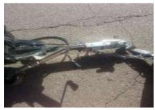
when pulling into Costco to get fuel I heard a big CLUNK and then a dragging noise. With the luck of drunks and fools (and I had not been drinking) I had driven 27 miles at highway speed without the pin through the receiver. I recommend giving the ball a tug too, just to make sure it is in there right.
